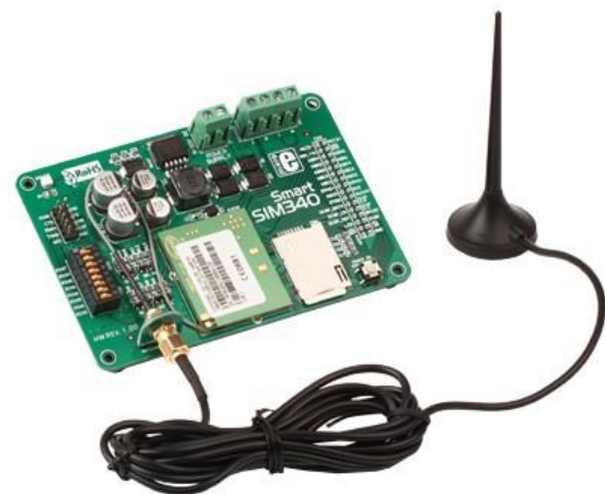
Figure 1: Sim340Z GSM Modem
