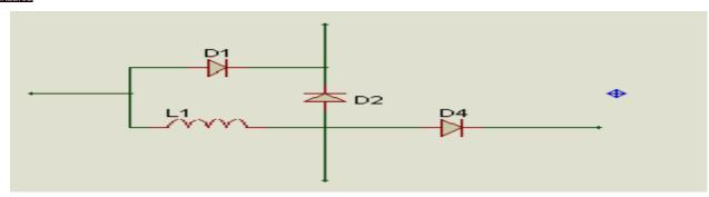
Fig.4. Switched Inductor (SL) Cell
