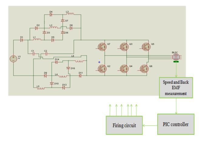
Fig.3.Generalized SL voltage-type Z-source inverter based BLDC drive
