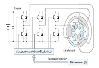
Fig. 2. Typical inverter drive system for a BLDC motor
