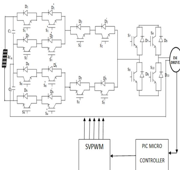
Fig.2 multilevel inverter
