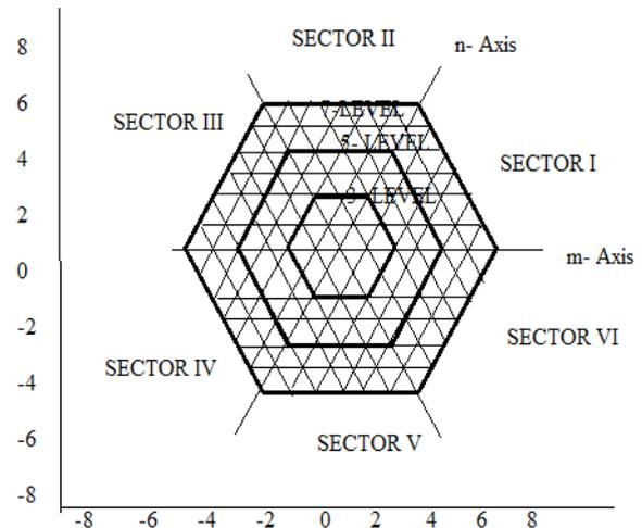
Fig.5 space vector for 7-level converter
