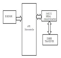
Fig-3. Block diagram of sensor node
