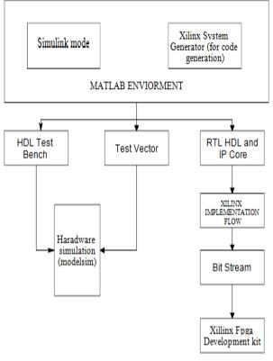
Figure: Block Diagram of System Generator
