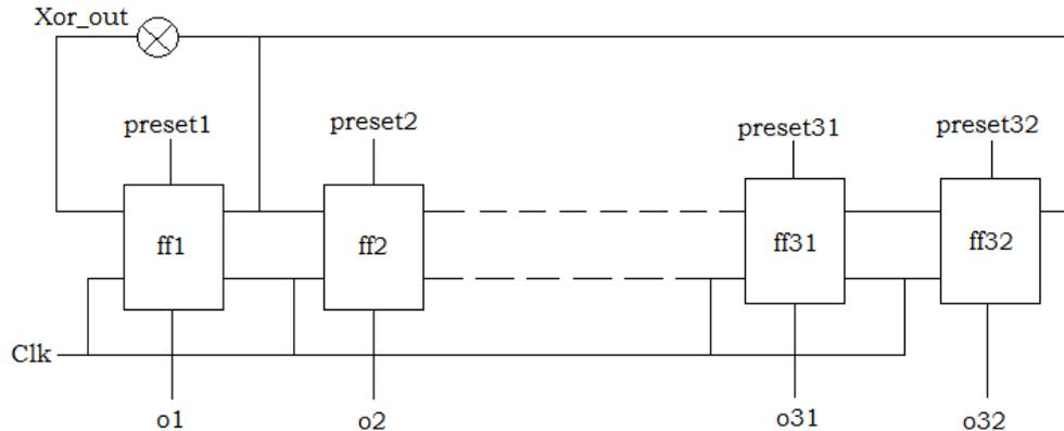
Figure1: Conventional Linear feedback shift register (LFSR)
