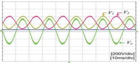
Fig 12.Output voltages of the boost inverter (V1, V2, and Vo) and dc input voltage, Vin
