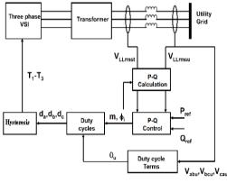
Fig 8. Block diagram of the overall control system of the inverter
