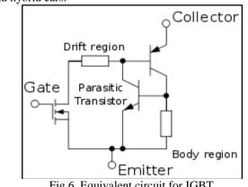
Fig 6. Equivalent circuit for IGBT
