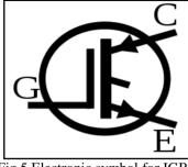
Fig.5.Electronic symbol for IGBT
