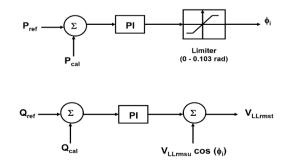
Fig 9. Control Diagram for Real and Reactive Power
