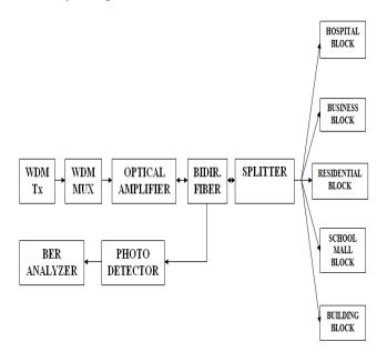
Fig 1 WDM Optical Network Simulation Model
