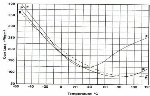
Fig.1 Loss Curves for the Different Core Materials
