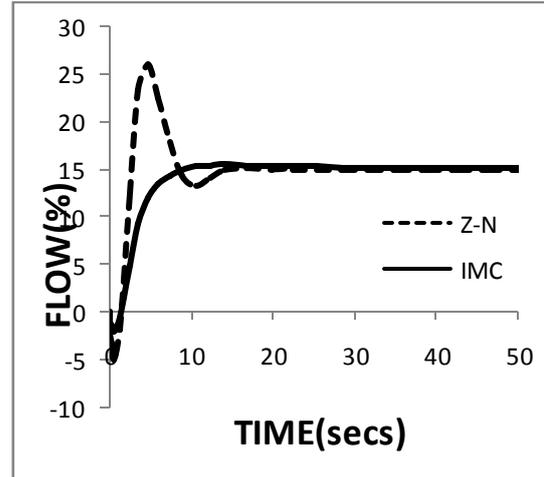
Fig. 3. Comparison of controllers in flow process
