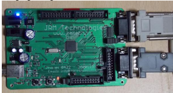
Fig. 4 LPC2148 microcontroller development board
