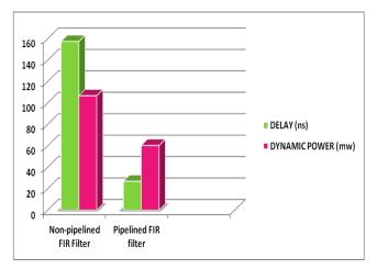
Fig. 6 Delay and Power analysis of FIR filter using Radix-4 multiplier.
