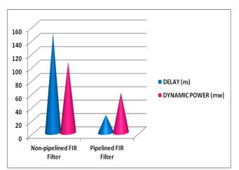
Fig. 7 Delay and Power analysis of FIR filter using Radix-8 multiplier.
