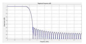
Fig. 3 FIR digital low-pass filter magnitude response
