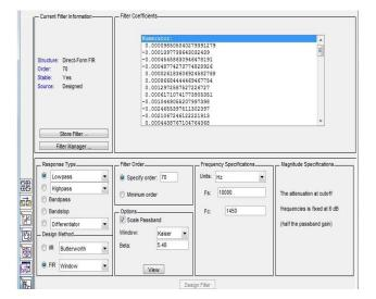
Fig. 1 FIR digital low-pass filter parameters.
