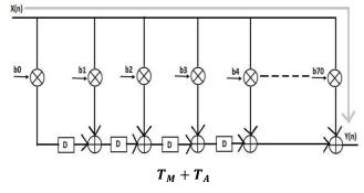
Fig. 4 Seventy-one tap pipelined FIR structure.
