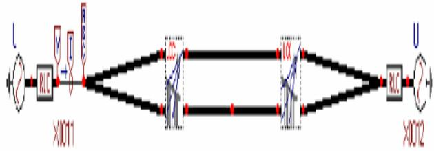
A single line diagram for the protected transmission line (T.L) is illustrated in Figure. It consists of two circuits of 80 km length, 66 kV voltage level and 2 GVA short circuit level.
