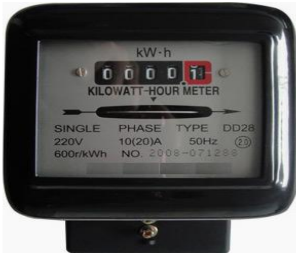
Figure.1 Traditional energy meter
