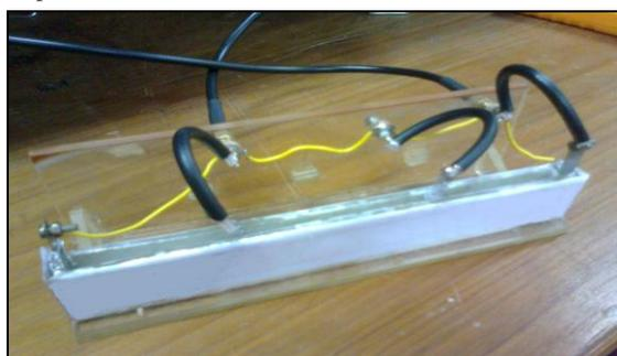
Fig. 1: Four probe impedance measurement cell
