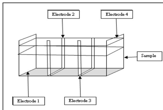
Fig.2: Schematic of the measurement cell
