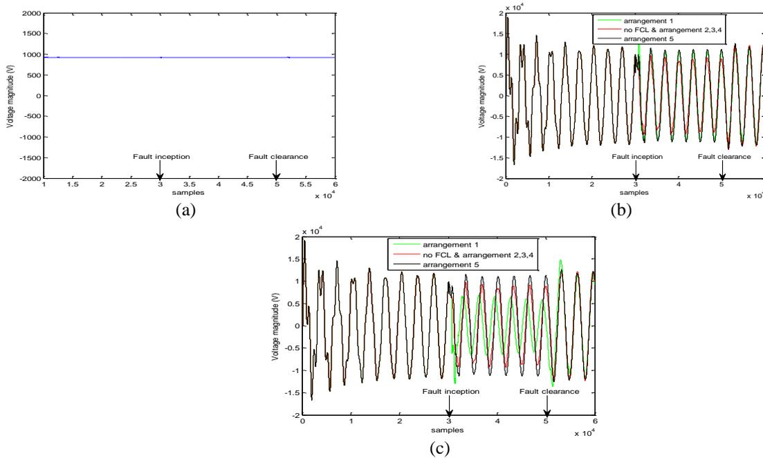
Fig.8. Voltage at different parts for fault occurrence in AC microgrid without DG, (a) at the output of PV source (bus12), (b) at the output of interior station transformer (bus3), (c) at the output of wind farm (bus7)
