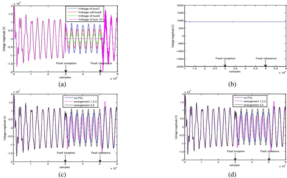
Fig.6. Voltage at different parts for fault occurrence in AC microgrid, (a) at the busses 7, 8, 9,10, (b) at the output of PV wind farm (bus 12), (c) at the output of the interior station transformer (bus3), (d) at the output of wind farm (bus7)
