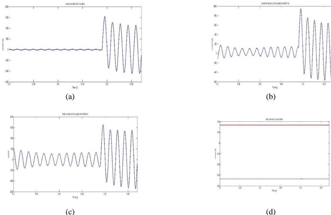
Fig.2. fault current in different parts of the network (a) in the fault position, (b) in the output of interior station transformer, (c) in the output of wind farm, (d) in the output of PV farm
