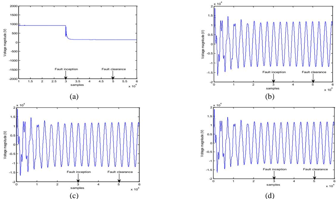
Fig.7. Voltage at different parts for fault occurrence in DC microgrid, (a) at the output of PV farm (bus12), at the output of interior station transformer (bus3), (c) at the output of wind farm (bus7), (d) at bus 5 in traditional grid
