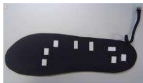
Fig. 3. Placement of sensors
