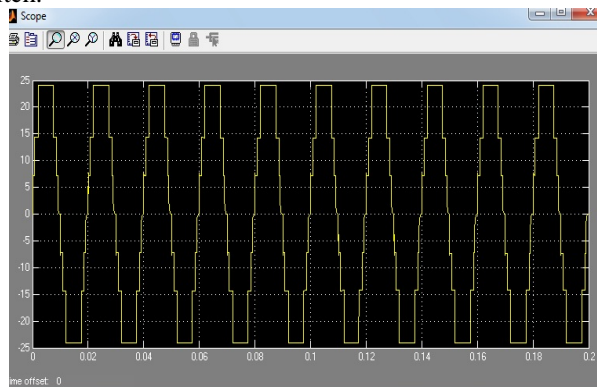
Fig.3 7 level inverter output waveform in Scope
