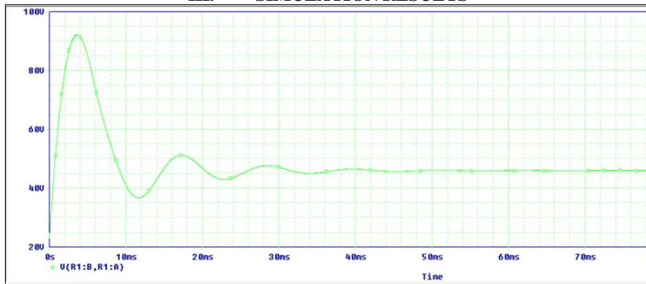
Fig 4: Output voltage of Interleaved boost converter
