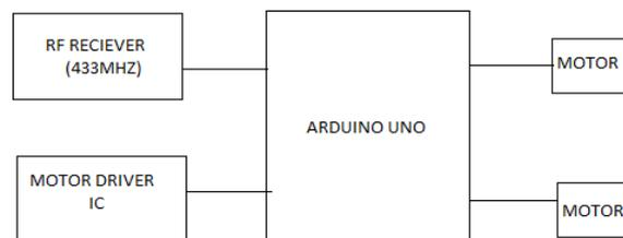
Fig. 5 Interfacing RF Receiver with Arduino
