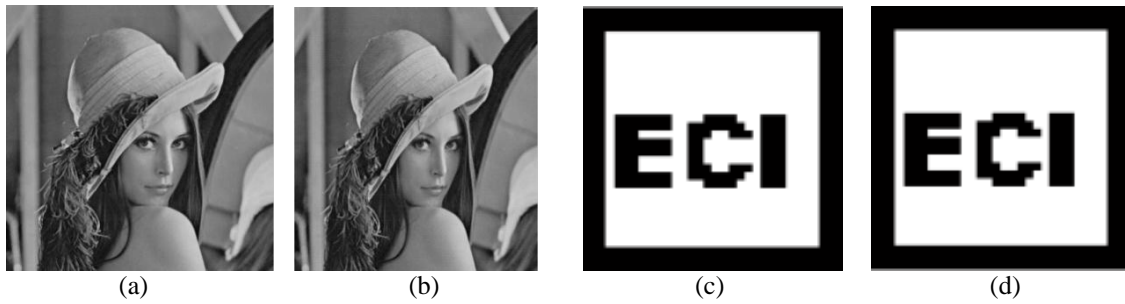
Fig.5( a) Host image (512x512), (b) Watermarked image, (c) Original watermark, (d) Extracted watermark without attack (NC=1)
