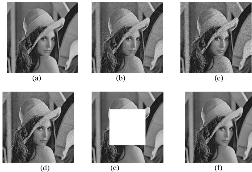
Fig.6 Watermarked “Lena” image distorted by different attacks (a) JPEG (Q=50), (b) Salt & pepper noise, (c) Speckle noise, (d) Gaussian noise, (e) Cropping, (f) Median filtering
