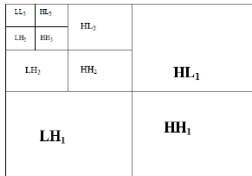
Fig.1 Three phase decomposition using DWT
