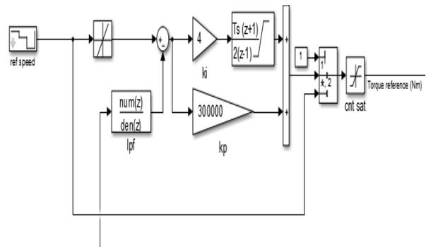
Fig.7 Simulink model of speed controller
