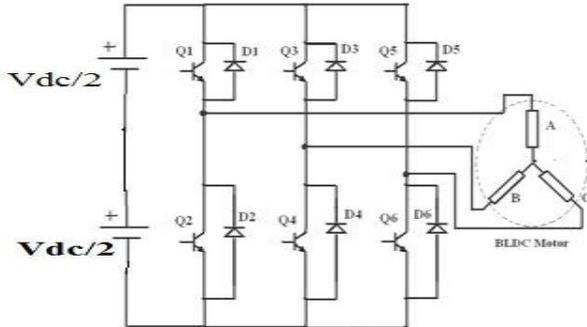
Fig. 3. Two level inverter fed BLDC motor
