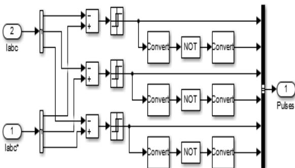
Fig.5 Simulink model of hysteresis current controller
