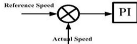
Fig.6 Speed controller block diagram
