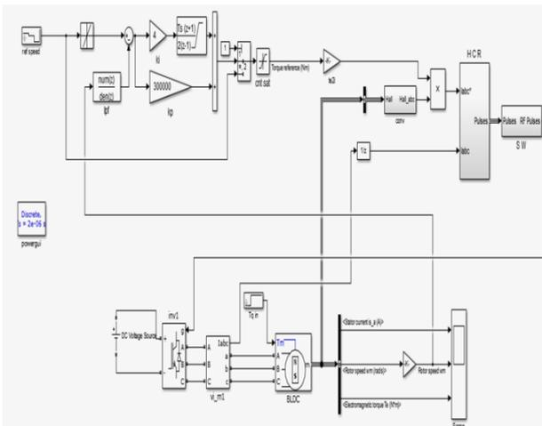
Fig. 9 SIMULINK model of BLDC motor drive without Hysteresis current controller loop
