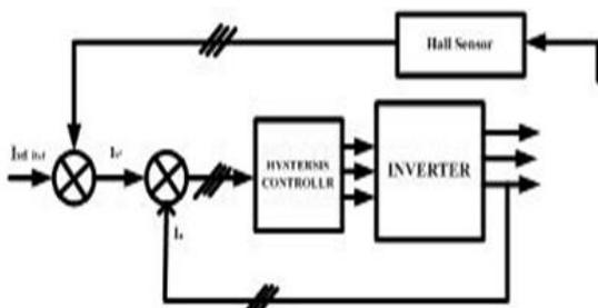
Fig.4 Block dia of hysteresis current controller
