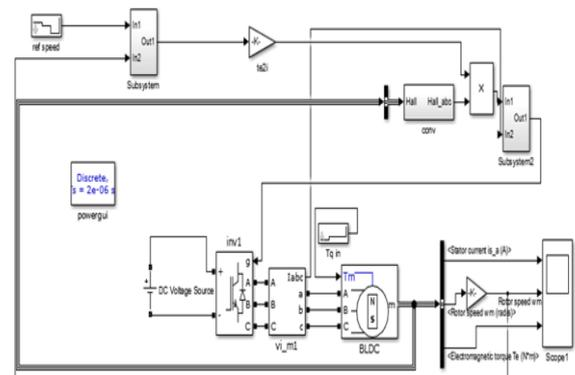
Fig. 8 SIMULINK model of BLDC motor drive without Hysteresis current controller loop.
