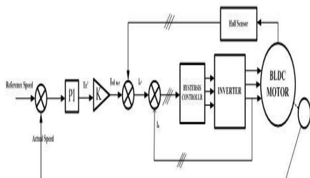
Fig. 2 Schematic of closed loop Two Level Inverter fed BLDC drive with Hysteresis Current controller loop
