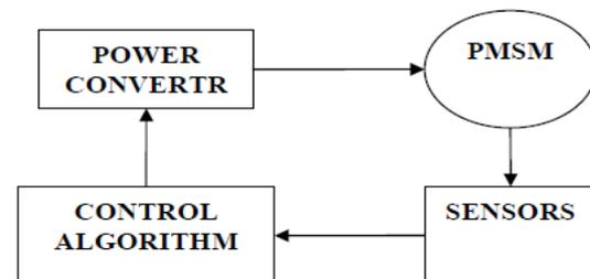
Fig.1 Block Diagram of Bldc motor control
