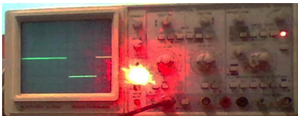
Fig12. Generation of PWM according to INC logic
