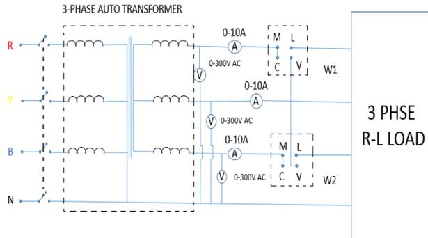
Fig.1:- Simplified electrical system of measurement of electrical parameters without SVC
