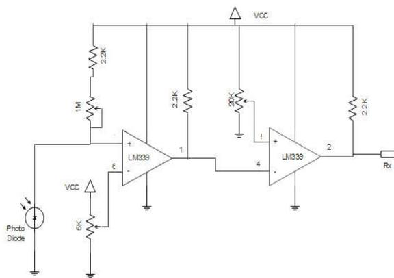
Fig. 5 Photo diode receiver circuit for Li-Fi
