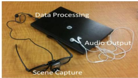
Fig.3. Snapshot demo system including three functional Components for Scene capture, data processing, and audio output.
