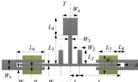
Fig. 4 - Structure of the SISLR in ref [4]
