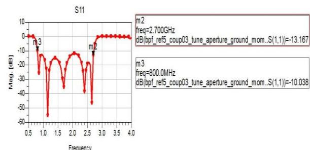
Fig. 13. The input return loss (S11) of the proposed wideband Bandpass filter.
