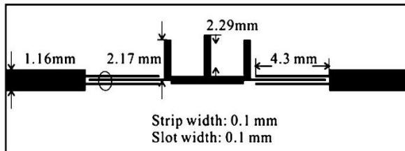
Fig. 2 Configuration of the proposed UWB BPF based on stub-loaded MMR in ref [2].
