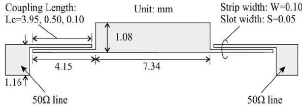
Fig. 1. Schematic of the compact Microstrip-line UWB Bandpass filter
