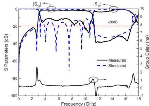
Fig 9 Simulated and measured frequency responses of fabricated UWB BPF.
