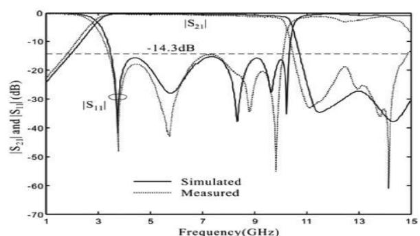
Fig. 7- Simulated and measured frequency responses of the optimized UWB BPF in ref [2]
