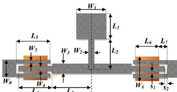
Fig. 5 UWB Bandpass filter in ref [5]
