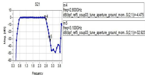
Fig. 12. The output gain (S21) of the proposed wideband Bandpass filter.
