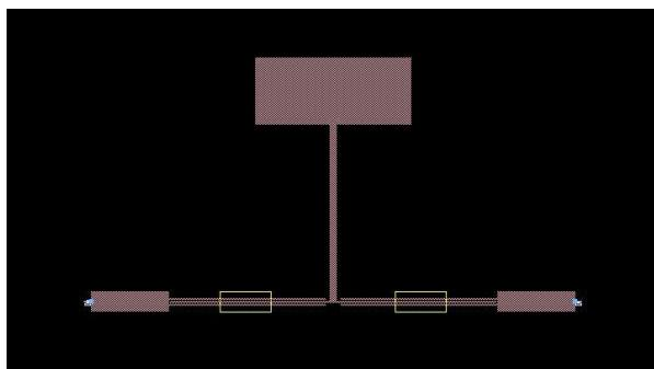
Fig. 11. The layout of the proposed wideband Bandpass filter.
