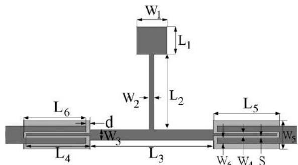
Fig. 3(a): Configuration of the UWB SISLR in ref [3]
