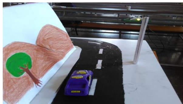
Fig. 12. Final output of sensor based accident prevention system by glowing of LED light.
