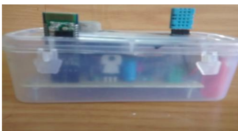
Fig. 3 Developed Node along with Bluetooth module
