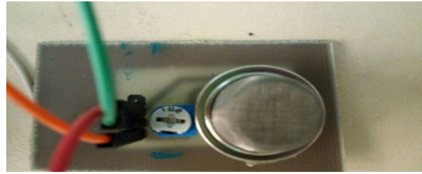
Fig.3.2 MQ135 along with signal conditioning (NH3 sensor)
