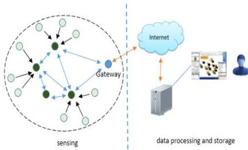
Fig. 1 Wireless sensor network components
