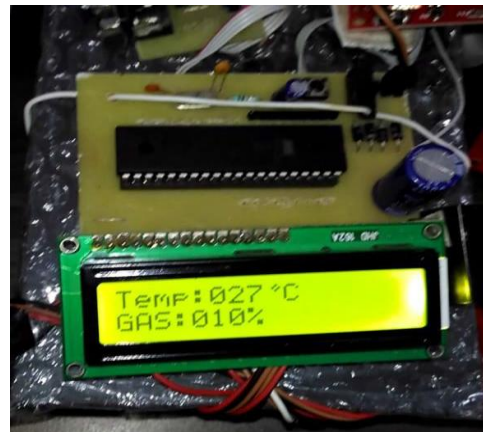
Fig.5 – Slave Robot displaying its own data
