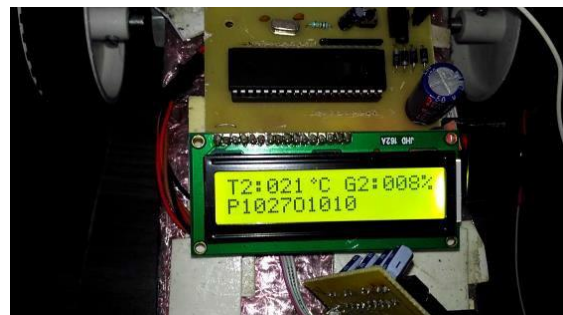
Fig.6 – Master Robot displaying the data of itself as well as the slave
