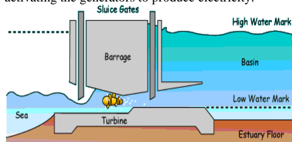
Fig. 5: Relationship between sea, turbine, basin, barrage and sluice gates
