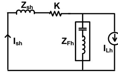
Figure 2 Harmonic equivalent circuit of SHAPF
