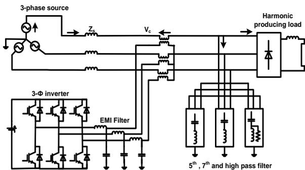
Figure 1 Series Hybrid Active Power Filter configuration
