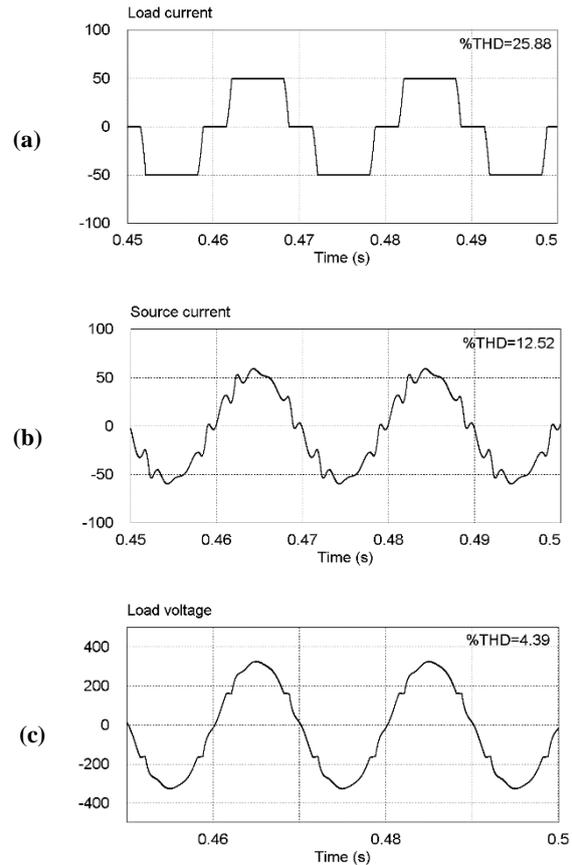
Figure 4 Simulation waveforms of the system with only passive filter: (a) Load current (b) Source current (c) Load voltage
