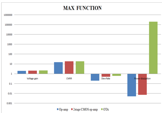
Fig 8 Comparison of MAX operator in terms of electrical parameters
