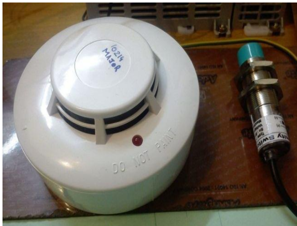
Fig. 2. Digital Smoke Sensor alongside with Proximity Sensor (right)
