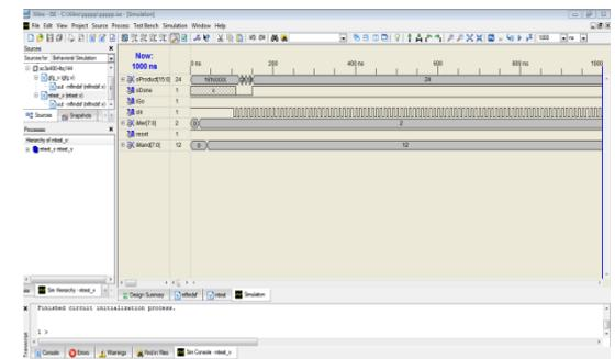
Fig 3: Output waveform for Radix 8 Booth multiplier
