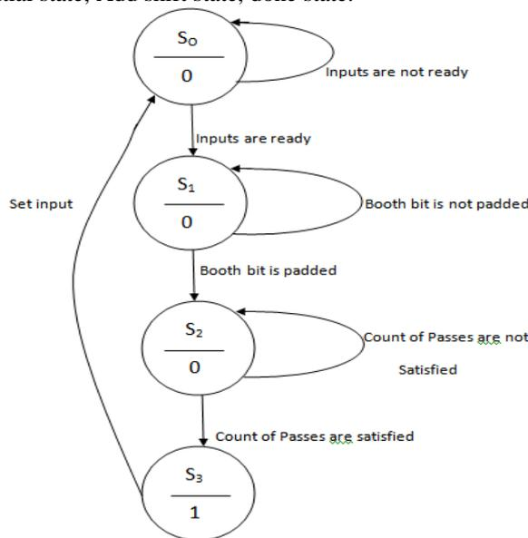
**Wait for Go state:** This state checks for the availability of the inputs for Radix 2 Booth multiplier. If the inputs are ready, the next state i.e initial state is activated and if the inputs are not ready then this state will be continued until the inputs are given by the user.
