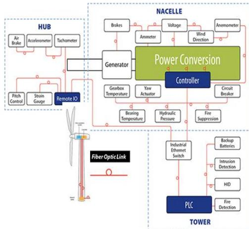
Fig.5. Fibre Optic Control Networking in a wind turbine.
