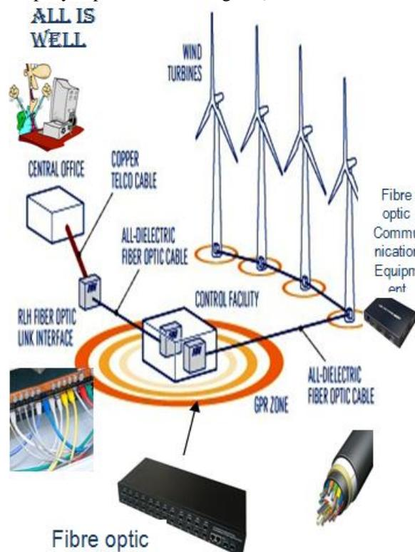
Fig.6 Typical Fibre Optic Network in Onshore Wind Farm
