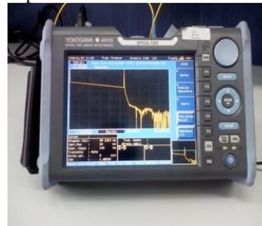
Fig.9 Optical Time Domain Reflectometer Source: [http://en.wikipedia.org/wiki/Optical\\_time-domain\\_reflectometer](http://en.wikipedia.org/wiki/Optical_time-domain_reflectometer)
