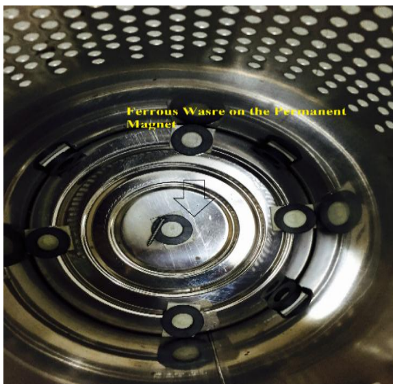
Fig.8. Base of the metal dustbin with permanent magnets to separate ferrous wastes
