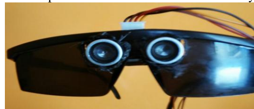
Figure 7: Ultrasonic Spectacle with HC-SR04 ultrasonic sensor
