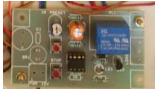
Figure 6: 555 timer used as a water detector
