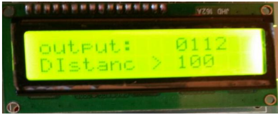
Figure 9: Distance displayed on the LCD screen
