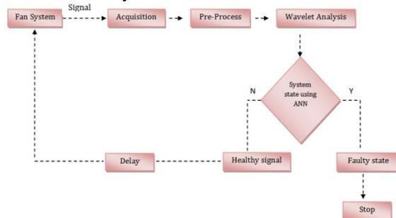
Fig. 2 Block diagram of fan fault diagnosis system
