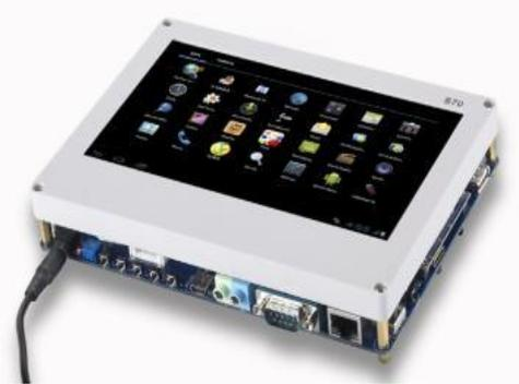
Fig.12 ARM11 dev. Board with TFT LCD
