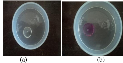
Figure 5: Phenolphthalein doped glass in (a) acid medium & (b) alkali medium
