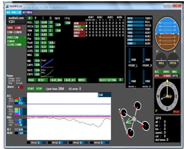
Fig. 3 MultiWii configuration interface (GUI)
