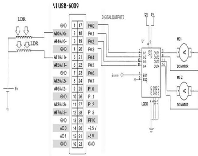
Fig.3. Solar Tracking Circuit
