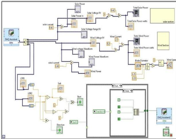
Fig. 5. Block Diagram in LABVIEW™ with use of DAQ Assistant (False)
