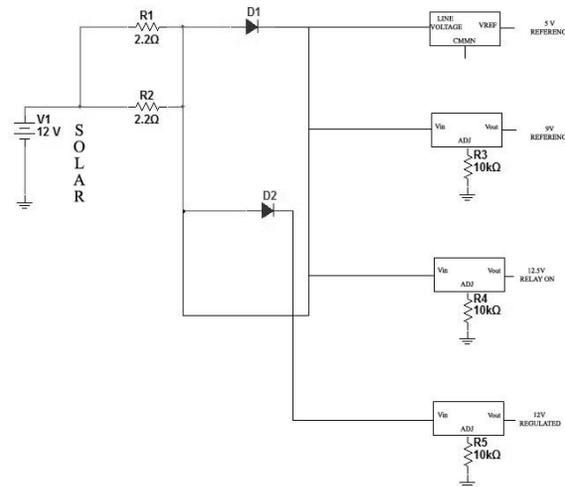
Fig. 2. Solar Power Generating and Regulating Circuit
