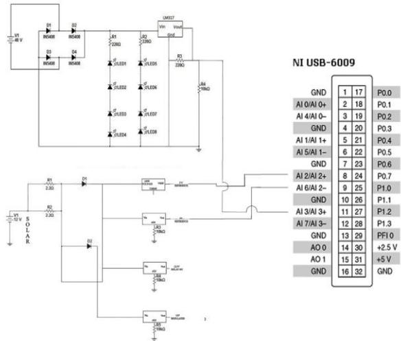
Fig. 4. Hybrid Power Generating System with NI USB 6009 DAQ
