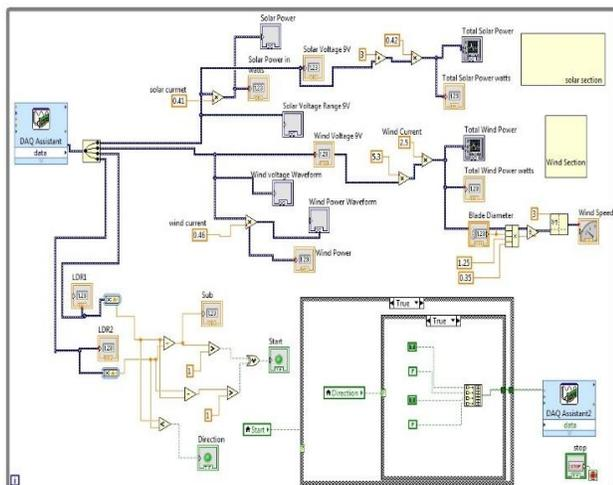
Fig. 6. Block Diagram in LABVIEW™ with use of DAQ Assistant (True)
