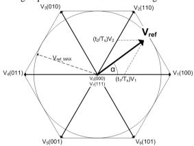
Figure-7 Space vector diagram for 2-level inverter
