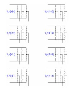
Figure-4 The eight inverter voltage vectors (Vo to  $V_7$ )
