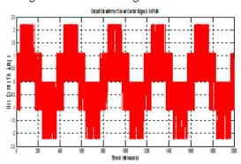
Figure-15.7-Line current without filter
