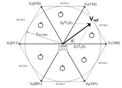
Figure-13 Space vector diagram for two level inverter
