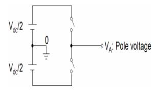
Figure-1 (a) circuit model of a single phase inverter
