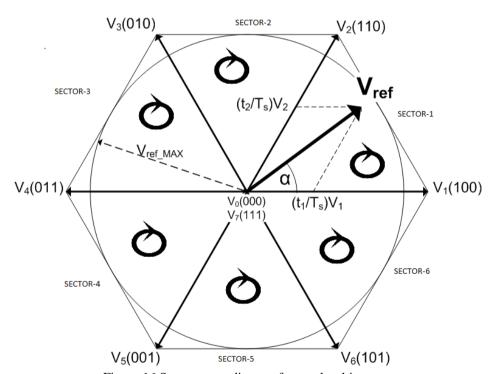
Figure-16 Space vector diagram for two level inverter
