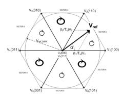
Figure-7.1 Space vector diagram for two level inverter
