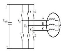
Figure-2 Three phase voltage source inverter with a load and neutral point
