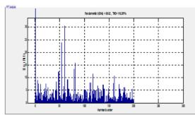
Figure-15.13-Line voltage THD without filter
