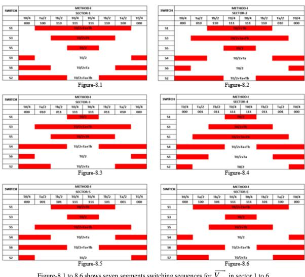
Figure-8.1 to 8.6 shows seven segments switching sequences for  $\overrightarrow{V_{ref}}$  in sector 1 to 6.
