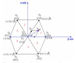
Figure-5 Basic switching vectors and sectors
