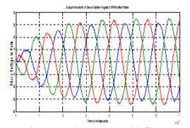
Figure-9.2-Phase voltage with filter
