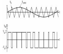
Figure-1 (b) pulse width modulation
