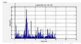
Figure-12.9-Phase voltage THD without filter
