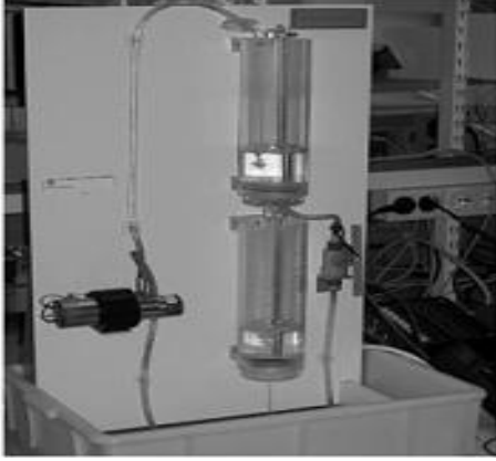
Figure 1 The cascaded two tank process
