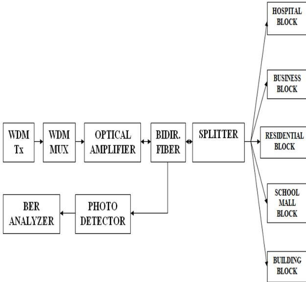
Fig 1 WDM Optical Network Simulation Model
