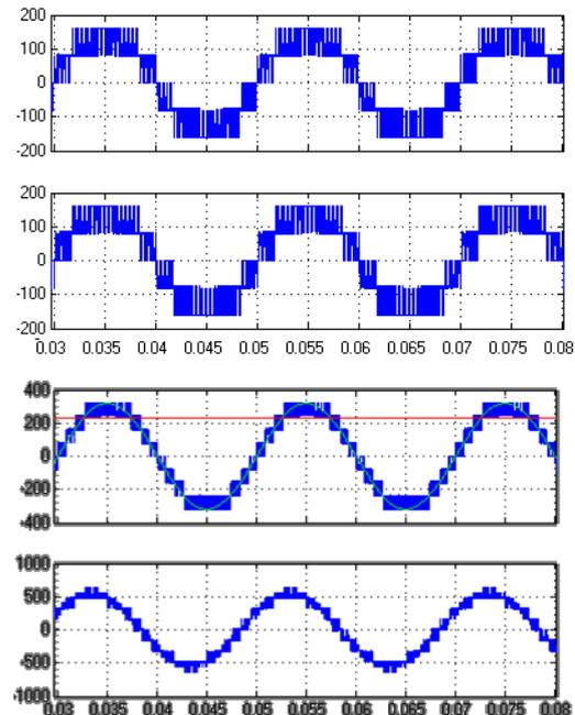
Fig. 8: Output voltage of TCHB inverter (a) Cell 1 output voltage & Cell 2 output voltage. (b) Phase & Line voltage.
