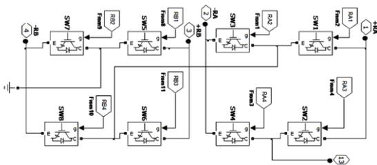
Figure 3: Cascaded H-bridge multi-level inverter limb per phase
