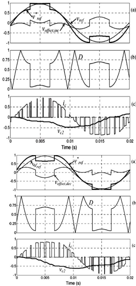
Figure 7: (a) Offset voltage to vary the midpoint capacitor voltage and the corresponding voltage reference, (b) duty cycle, (c) midpoint capacitor current and voltage.
