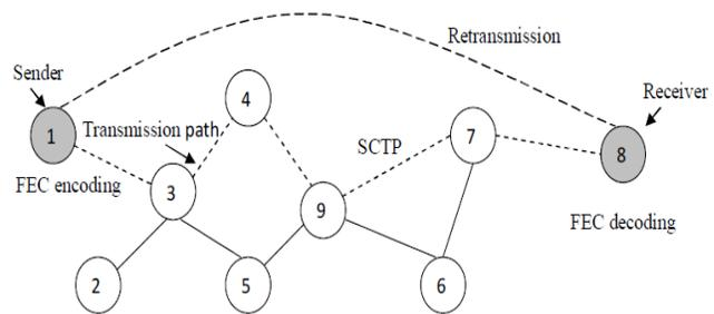
Fig.3. Sctp and FEC based Loss Recovery Technique
