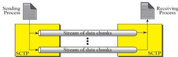
Fig.2. Multistreaming using SCTP
